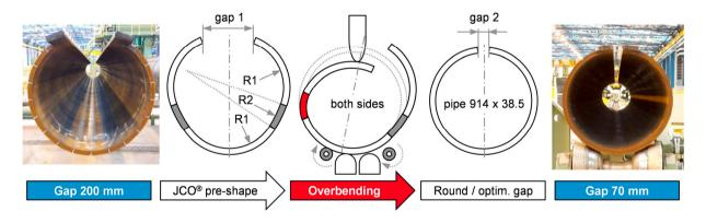
Fig 2. Pipe closing process with special pre-shape
