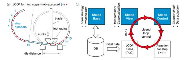
Fig. 1. JCO<sup>®</sup> forming process (a), interaction of the Shape modules for process control (b)
