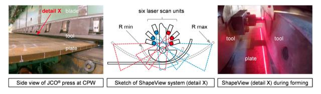
Fig. 3. ShapeView system integrated into the blade during forming
