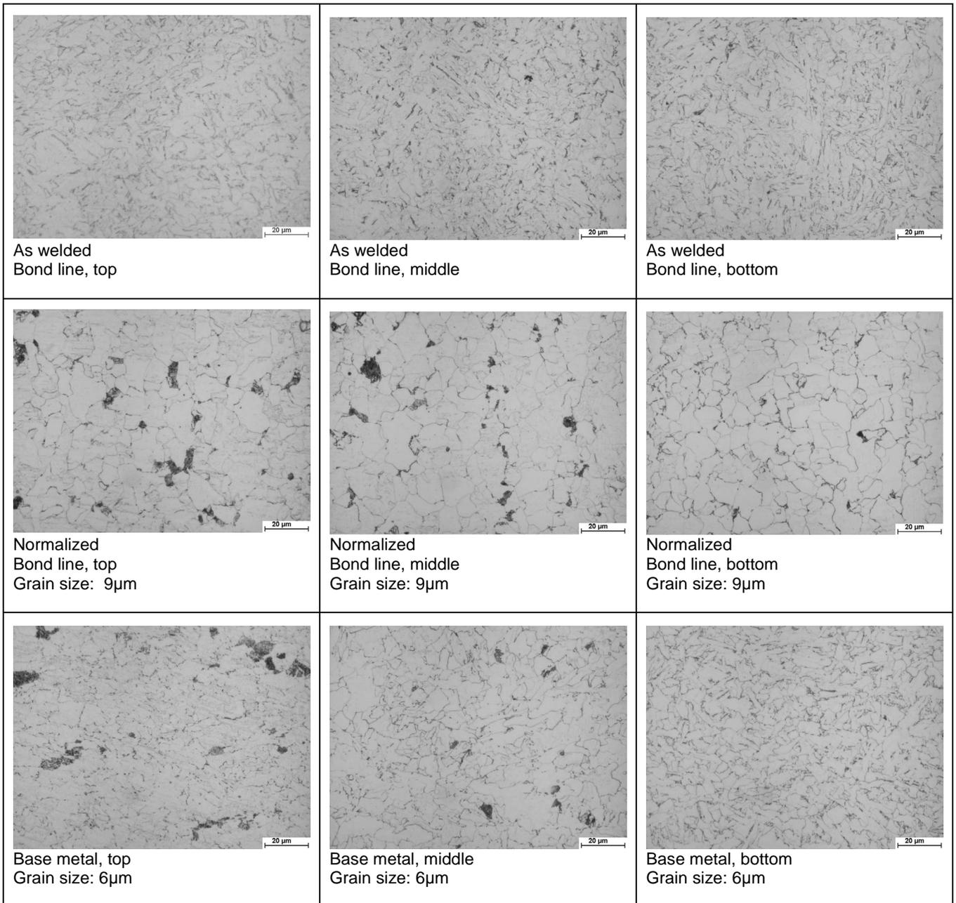
**Figure 4: Microstructure of as welded, normalized and base metal 25mm samples. Average grain size measured with image analysis. Samples were polished and etched with 2% nital.**
