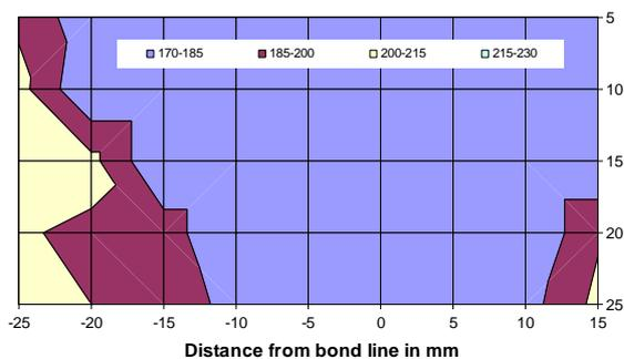
**Figure 5: HV10 hardness mapping of the weld seam cross section**
