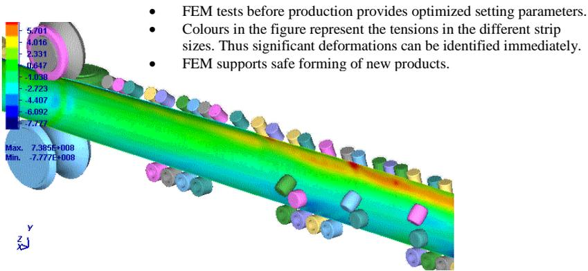
Figure 2: FEM Integrated Analysis for forming optimisation
