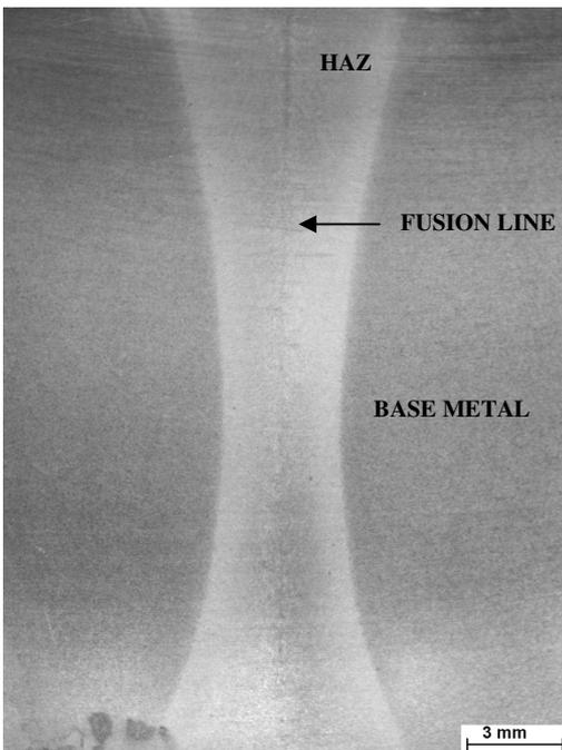
Figure 3: Cross section specimen of the weld (24" X 25mm X60, as weld condition)
