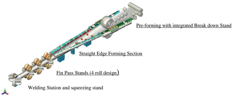
Figure 1: General Forming Layout – Main Components of the Forming Mill
