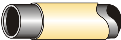
Fusion bonded epoxy (single and dual layer) Epoxy lined or internally epoxy coated
